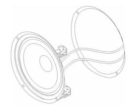
**STEP C.** Before sliding the speaker into the frame cutout hole, be sure to loosen the dog-ear clamps. Then, carefully place the speaker into the frame cutout hole.
